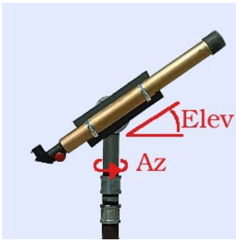
Alt-azimuth Mount showing elevation and azimuth (horizontal axis)
